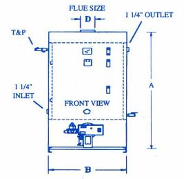
NOTE: STANDARD GAS PRESSURE REQUIREMENTS: Natural Gas 7 - 11 inches w.c. Required @ Heater Propane Gas - 14 inches w.c. Required @ Heater Gas trains for higher and lower pressures available. Consult factory.
